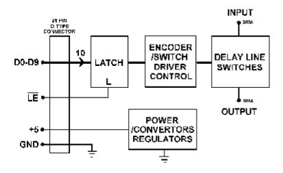
The delay line consists of passive GaAs microwave transfer switches. The switch network series resistance losses are matched with shunt resistance to ground for improved wide-band matching.
